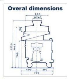
MAIN USES: Vibrating screen for solids and liquids sleving, filtering, separating, dedusting
